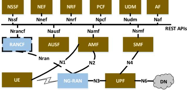
Figure 1: Envisioned 5G functional architecture based on the 3GPP Release 15 including the proposed RANCF function. NG-RAN functions are marked in blue and 5GC functions in brown. A breakdown of the NG-RAN functions is illustrated in Fig. 2
