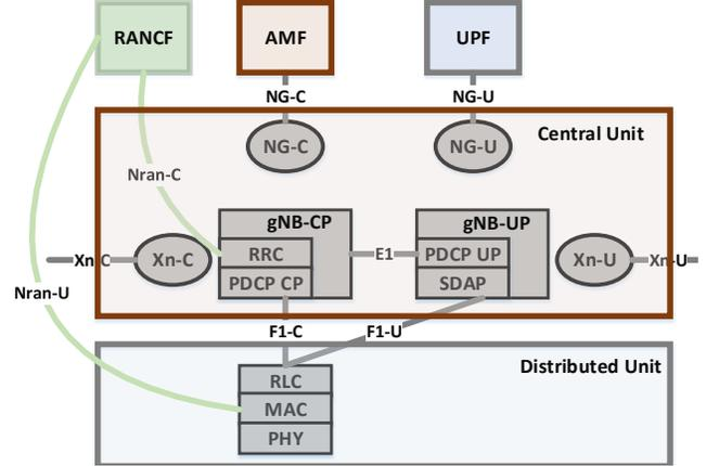
Figure 3: Envisioned NG-RAN functional architecture based on a separation of functions between distributed units, centralized units and an SD-RAN controller (RANCF). NG-C and NG-U are interfaces to the 5GC. Proposed interfaces to the proposed RANCF are Nran-C and Nran-U.
