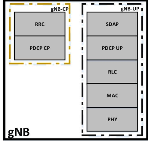
Figure 2: Overview of NG-RAN functions mainly realized in the 5G gNB (base station). We distinguish between control plane (gNB-CP) and user plane (gNB-UP) functions. Interfaces to the 5GC functions are shown in Fig. 1
