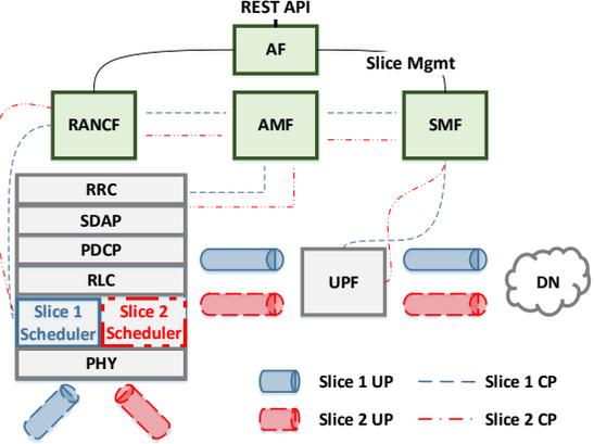
Figure 4: Illustration of the interaction of 5G functions and RANCF to support end-to-end network slicing. Dashed lines show control information flows. Tube shapes represent isolated user plane slices from the UE through the 5G RAN and core to the Data Network (DN).
