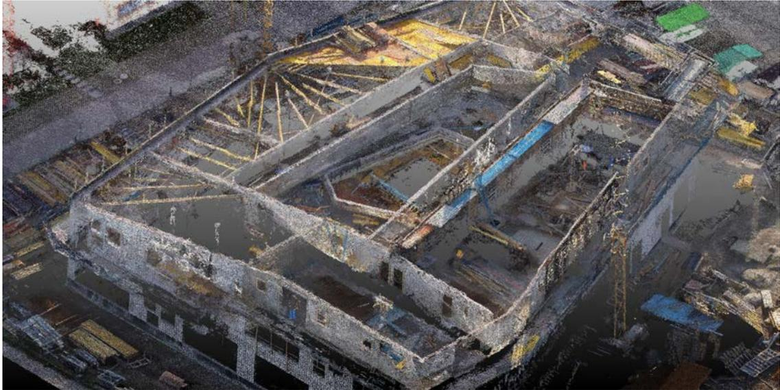
**Figure 52** Occluded construction elements in generated point cloud caused by scaffolding, formworks, existing elements and missing information during the reconstruction process
