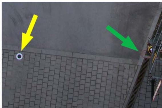
(a) Photogrammetric marker (yellow arrow) and surveying point (green arrow)
