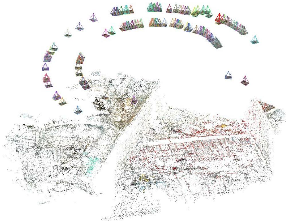
**Figure 14** Reconstruction process using VisualSFM with visualized camera positions including their viewing directions (camera cone).
