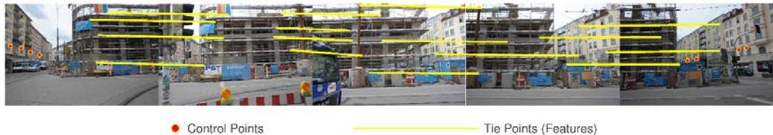
**Figure 18** Image orientation process using control points and tie points
