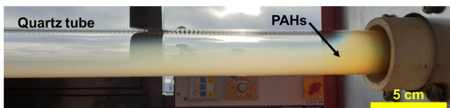
**Figure 3.6:** A photograph of the quartz tube during a GC deposition process at the pump/exhaust side of the furnace. Polycyclic aromatic hydrocarbons are formed in the gas phase and condense as film on the inner surface of the cooler quartz tube.
