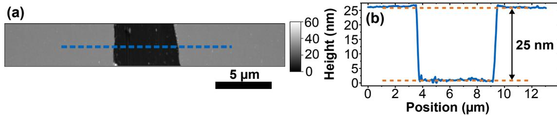
**Figure 2.18:** Thickness of a GC film measured with an AFM. (a) The surface morphology at a point where a narrow strip of carbon was scratched away with a test needle. The underlying silicon nitrite is almost undamaged. (b) The measured profile along the dashed line indicates a steep step with a height of 25 nm.
