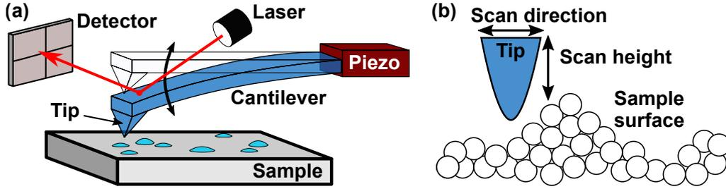
**Figure 2.17:** The schematic working principle of an AFM. (a) In tapping mode, an oscillating cantilever is moved in proximity across a sample. The interaction of the tip with the surface of the sample is sensed by a detector with laser light reflected from the cantilever. (b) A feedback loop alters the scanning height of the tip if a change in the surface profile, indicated schematically by atoms, is detected.
