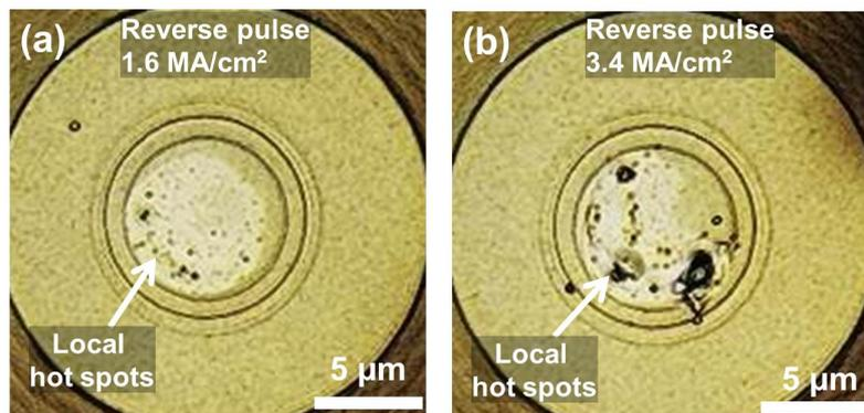
**Figure 5.1:** Micrographs of failed C-Si diodes after being stressed with a single current pulse applied in the reverse direction of the diode. A current density of (a)  $1.6 \text{ MA/cm}^2$  and (b)  $3.4 \text{ MA/cm}^2$  was used. A damage is clearly visible as burn marks on the 200 nm thick top metallization, which were caused by very localized high temperature hot spots. The higher the current density, the more severe is the damage.
