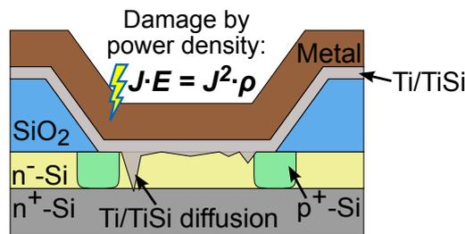
**Figure 5.5:** A schematic cross-section of a simplified TiSi-Si Schottky diode where a high current pulse was applied. The Joule heating (see Eq. 1.4) forces Ti or rather TiSi to diffuse into the n<sup>-</sup>-Si epitaxial layer, which could even reach the highly doped substrate.
