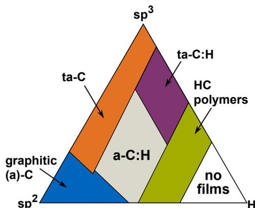
**Figure 3.1:** (a) Ternary phase diagram of different amorphous and disordered carbon-hydrogen alloys. The materials are classified on their ratio of  $sp^2$  and  $sp^3$  hybridized C bonds and the amount of incorporated H. Adapted from Ref. [269].
