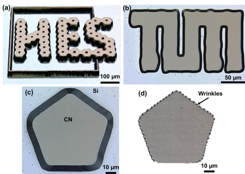
**Figure 3.20:** Micrographs of patterns etched with KOH using CN as etching mask. (a) shows a slightly tilted structure in a 3D view. The height is 6  $\mu\text{m}$  and is shown enlarged by a factor of six compared to the indicated scale bar. (b) and (c) show a top view of two patterns indicating facets in the silicon. (d) shows the CN film from (c) with height information (enlarged by a factor of 20) to highlight the wrinkles at the edges where the carbon was undercut.
