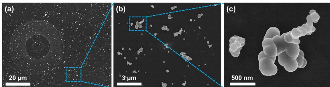
**Figure 3.11:** SEM images of a surface after a GC deposition process from  $C_2H_4$  in no-flow conditions ( $1000\text{ }^\circ\text{C}$ , 42 mbar). (a) shows an image in the region of the diode that is speckled with soot particles. Scans with higher magnification in (b) and (c) show that individual particles conglomerate and form larger objects. The images were obtained at an acceleration voltage of 4 kV and a working distance of 7 mm.
