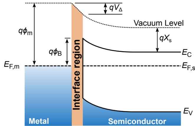
**Figure 2.9:** Energy-band diagram of a metal-semiconductor contact with a non-ideal contact. The interpretation of the interface region depends on the respective model and can be a layer caused by interface states or an interface specific region where a bond-polarization causes an interface dipole. Independent of the model, a potential drop  $V_{\Delta}$  occurs, leading to a change in the SBH.
