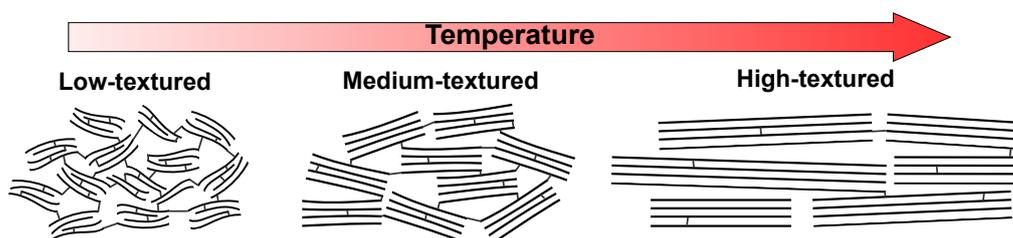
**Figure 3.3:** Schematic representation of the preferred orientation of deposited GC at different substrate temperatures after Ref. [280]. The carbon crystallites become larger and better orientated to each other at an increased temperature. It is further assumed that the defect density is reduced, which leads to a lower number of covalent bonds between the individual layers and crystal grains.
