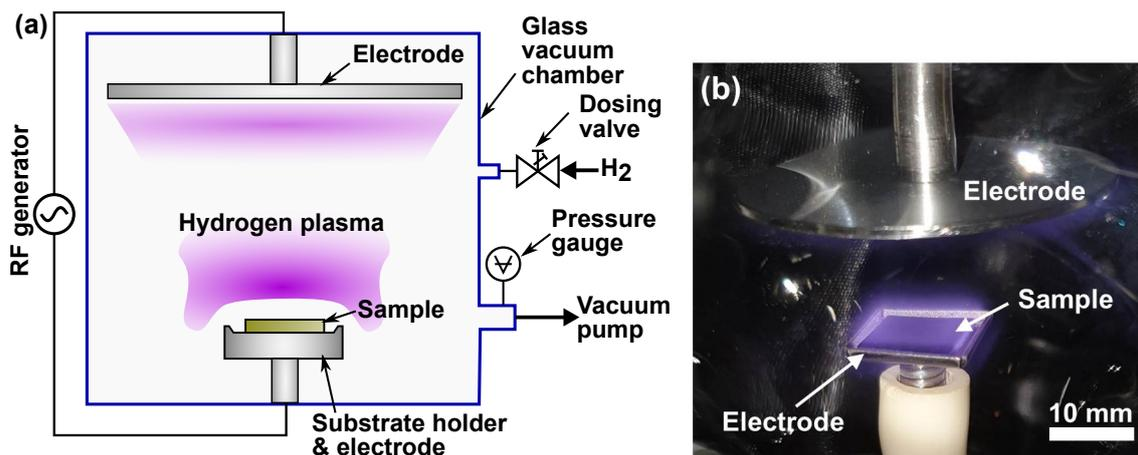
**Figure 3.23:** (a) A schematic representation of the CCP structure used for etching carbon with a hydrogen plasma. The pressure in the reactor can be adjusted by changing the gas flow with a needle valve. The photograph in (b) shows the real setup used, whereby the plasma is clearly recognizable around the sample.
