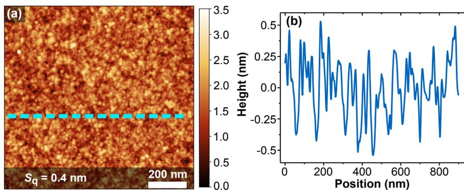
**Figure 3.9:** Surface roughness and corresponding height profile of a deposited GC film by pyrolysis from  $C_2H_2$  gas measured with an AFM. The film was grown at  $860^\circ C$  and 24 mbar for 9 min. (a) shows that the film is very smooth and does not show large particles (soot) or pits. (b) shows the surface profile along the dashed line. The average height is here set as zero height.
