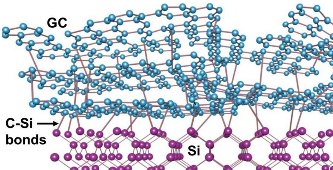
**Figure 1.12:** A schematic representation of a graphenic carbon to silicon contact (Si with (111)-surface). The individual GC sheets are not defect-free, thus not only  $sp^2$  hybridization occurs and cross-links (bonds) between the stacked planes at lattice imperfections are formed. Covalent bonds between C and Si atoms are also formed, whereas the total number of interlayer bonds and defects shown here might differ from a real film.
