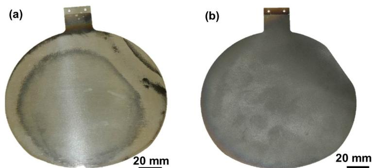
**Figure 3.16:** Photographs of different shutters after they were coated. In (a) the metal surface was polished and the carbon did not stick properly and could easily be wiped off. On the upper right part of the shutter is an arc visible because the shutter reached in the ‘open’ position slightly into the plasma. The shutter in (b) was glass bead blasted before it was sputtered with C on both sides while lying on the substrate plate. The part that protruded into the plasma was cut off.
