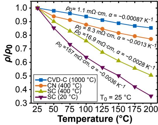
**Figure 4.10:** Measurement of the temperature-dependent relative electrical resistivity  $\rho/\rho_0$  of CVD-C deposited at 1000 °C, CN deposited at 400 °C and SC deposited at 400 °C and 20 °C, respectively.  $\rho_0$  is the initial resistivity at  $T_0 = 25$  °C. All of them feature an NTC  $\alpha$ , which was fitted for simplicity with a linear behavior over the measured temperature range. Taken from Ref. [MS19].
