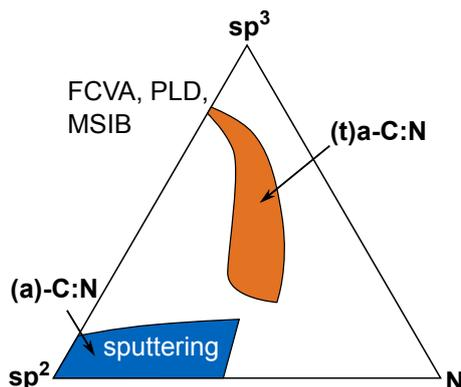
**Figure 3.13:** Ternary phase diagram of different amorphous carbon-nitrogen alloys. The materials are classified on their ratio of  $sp^2$  and  $sp^3$  hybridized C and the amount of incorporated N. Sputtering yields more graphitic carbon. Films with higher  $sp^3$  content (ta-C:N) are produced by filtered cathodic vacuum arc (FCVA), pulsed laser deposition (PLD) and mass selected ion beam deposition (MSIBD). Adapted from Ref. [296].
