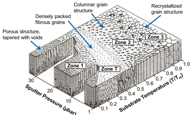
**Figure 3.14:** The structure zone model proposed by Thornton [297,299] for columnar thin films produced by sputter deposition. Three main and a transition zone between zone 1 and 2 are indicated. The relevant process parameters are the Ar pressure and the substrate temperature  $T$  (in Kelvin) which is normalized by the melting point  $T_m$  of the sputtered material. Reprinted from Ref. [297], with the permission of AIP Publishing.
