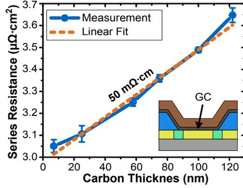
**Figure 4.3:** The area-normalized series resistance of the CVD-C-Si diode  $R_s$  as a function of the graphenic carbon thickness. All tested diodes have similar GC deposition parameters, only the growth time was altered, and the same metallization layers on top. The out-of-plane electrical resistivity is extracted to be 50 mΩ cm. Taken with permission from Ref. [MS17] © 2017 IEEE.
