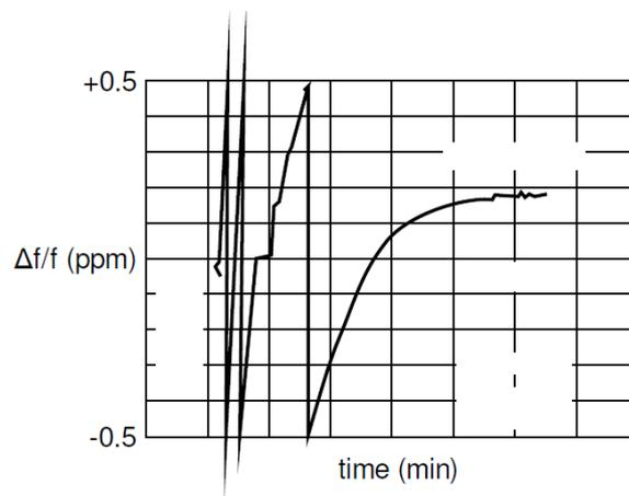
**Figure 4.** Frequency difference during the warm-up phase of the DW1000 crystal oscillator in parts per million (PPM) with respect to the time in minutes [15]. The figure is used with permission [15].
