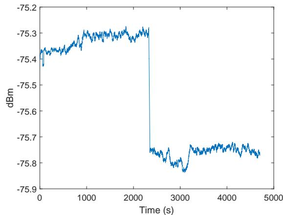
**Figure 5.** Signal power in dBm of the received blink message. The curve shows the filtered results of the received signal power over time, measured by the DW1000 chip. After 4600 measurements the transmitting signal power was reduced.
