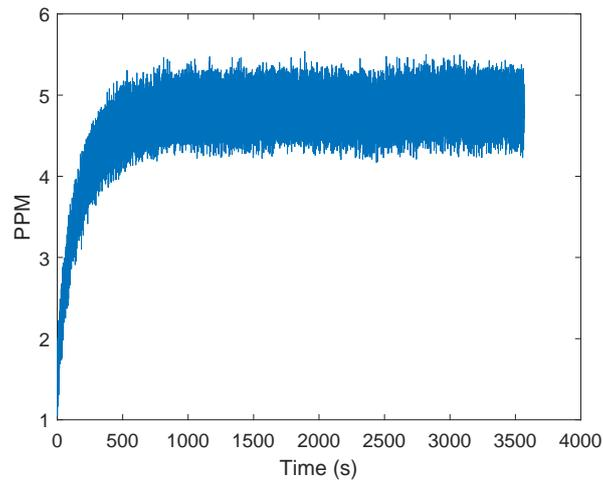
**Figure 2.** Frequency difference between the received carrier and the internal phase locked loop (PLL) in parts per million (PPM). The curve is obtained by reading the carrier integrator value of the DW1000 chips. The logarithmic increase of the curve is due to the warm-up of the crystal oscillator.
