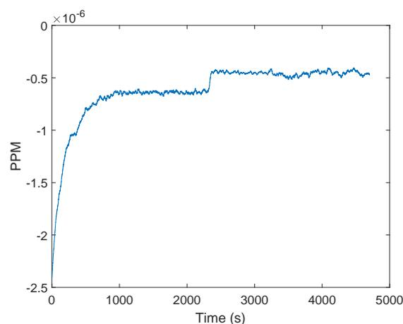
**Figure 6.** Filtered frequency differences between the received carrier and the internal phase locked loop (PLL) in parts per million (PPM) after changing the transmitting signal power after about 2340 s.
