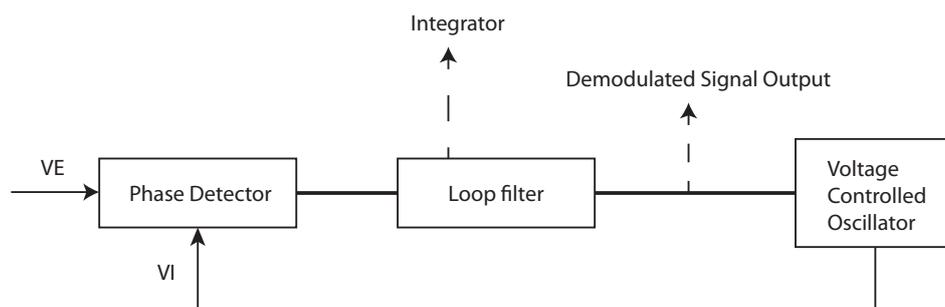
Figure 1. Example of the phase locked loop (PLL).
