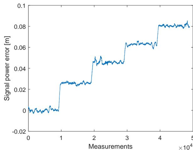
**Figure 15.** Filtered timestamp error changes due to the received signal power. The measurements have been obtained with a cable connection between the transceivers. The error is changing systematically with decreasing signal power.
