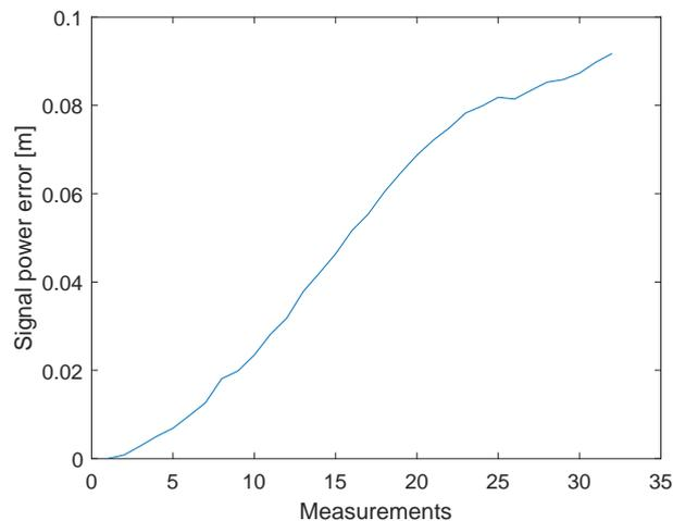
**Figure 17.** Filtered timestamp error changes due to the received signal power. The measurements have been obtained with a wireless connection between the transceivers. The error is changing with decreasing signal power.
