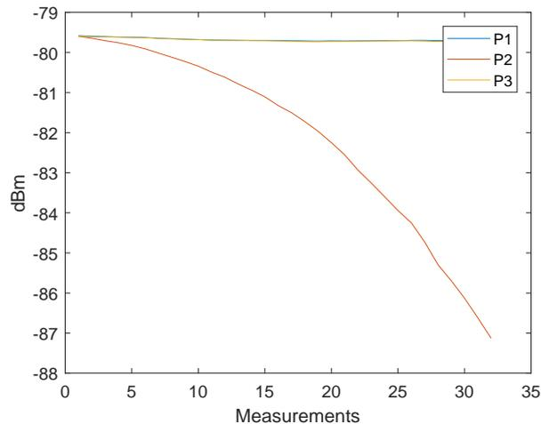
**Figure 16.** Filtered received signal power measurements of the three messages P1, P2 and P3. The measurements have been obtained with a wireless connection between the transceivers. The transmitted signal power of the second signal P2 is reduced with a step size of 0.5 dB, while the signal power for P1 and P3 remains constant.
