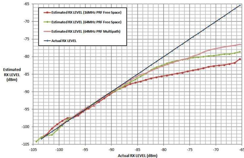
**Figure 13.** Measured received signal power at the DW1000 chip, with respect to the correct signal power. The blue line represent the reference line, every value of the x-axis has the same value on the y-axis. The other lines are the results of the estimated received signal power with different settings. The estimated received signal power equates the correct signal power for low signal strength [14].
