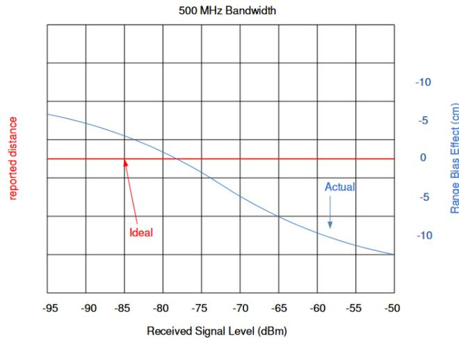
**Figure 12.** The effect of the received signal power on the distance measurement [15], used with permission. The red line represents the correct distance measurements. The blue line shows the range bias caused by different signal powers [15].
