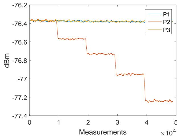
**Figure 14.** Filtered received signal power measurements of the three messages P1, P2 and P3. The measurements have been obtained with a cable connection between the transceivers. The transmitted signal power of the second signal P2 is reduced with a step size of 3 dB, while the signal power for P1 and P3 remains constant.
