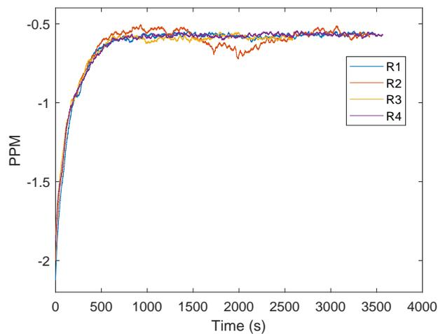
**Figure 3.** Filtered frequency difference between the received carrier and the internal phase locked loop (PLL) in parts per million (PPM). The colors represent different measurement obtained successively. It can be seen that the curves are deterministic.
