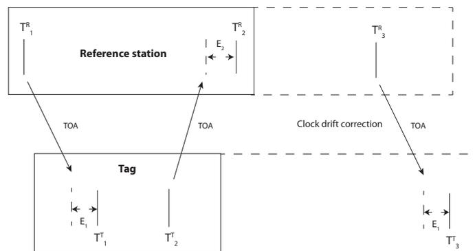
Figure 24. Two-way ranging with clock drift correction between reference station and tag.
