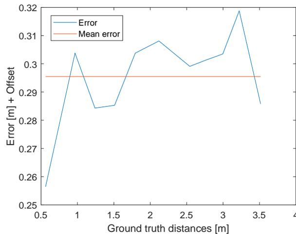
**Figure 25.** Difference between the measured distances obtained by two-way ranging and the ground truth distances in meter. The constant offset caused by the hardware delay is not compensated but is represented by the red line. The near most constant errors for different distances shows the power correction is correct.
