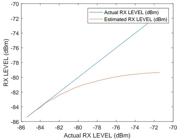
**Figure 19.** Estimated correction curve between the measured received signal power and the ideal signal power curve.
