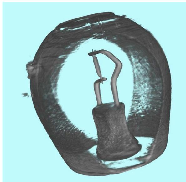
**Figure 16.** Cut-open 3D view of the optical CT of the light bulb.
