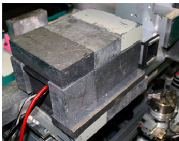
**Figure 5.** External shielding stacked.
