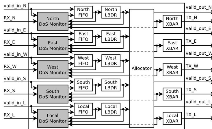
Figure 10. Proposed router architecture with Denial of Service (DoS) detection.
