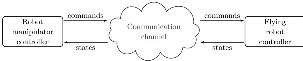
**Figure 1.6:** Communication channel with information directions.
