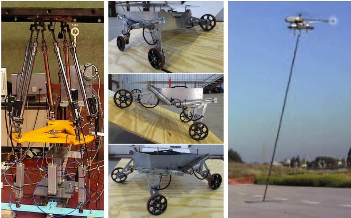
(a) Self-leveling landing platform presented by Campos et al. [9]. The lower part is a parallel robot with three DoF and pneumatic prismatic actuators. It simulates ship motion and is used for testing the so-called active helideck (upper part, six DoF and prismatic electrical actuators).
