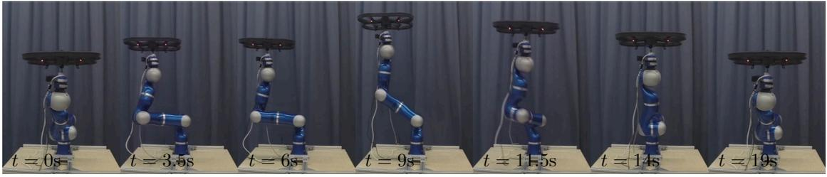
**Figure 4.4:** Picture sequence from the performed experiment with the controller from Section 4.2.5. The indicated time instants correspond to the plot in Figure 4.7. A short video is provided on-line [172] showing the robotic assistance system for flying robots and some of the conducted experiments. Copyright © 2016 IEEE [208].
