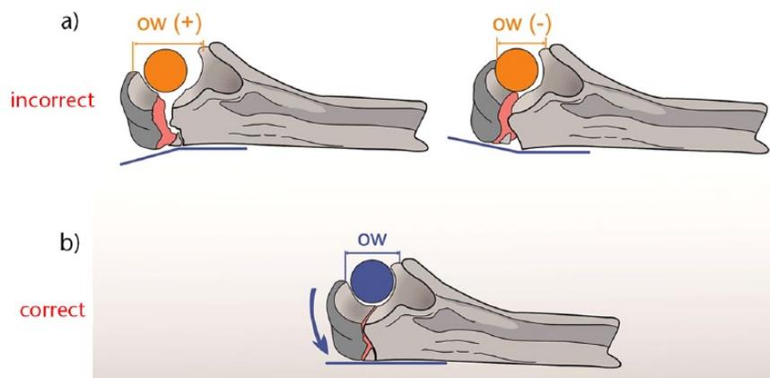
**Fig. 3** (a) incorrect reconstruction: constriction (left) or enlargement (right) of the olecranon width (OW) due to an incorrect dorsal alignment; (b) correct reconstruction.
