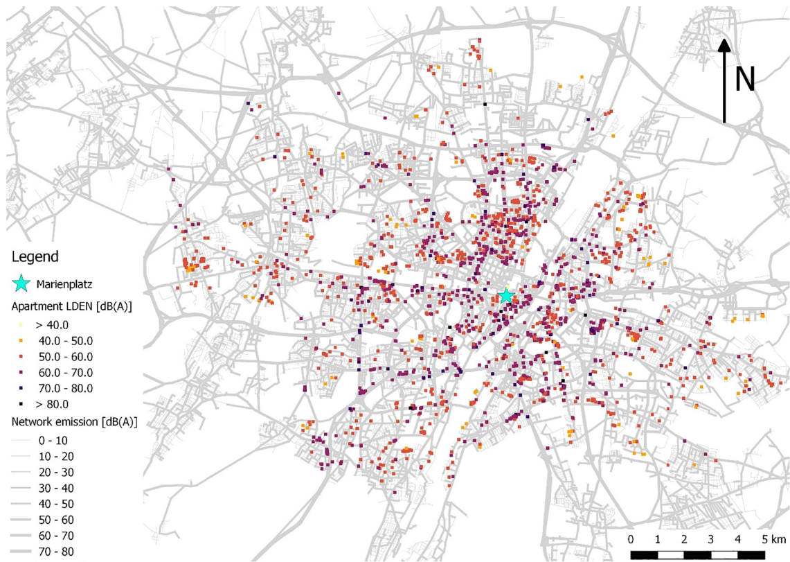
Fig. 5. Calculated network emissions for 8 AM peak hour and averaged daily immissions for apartments.
