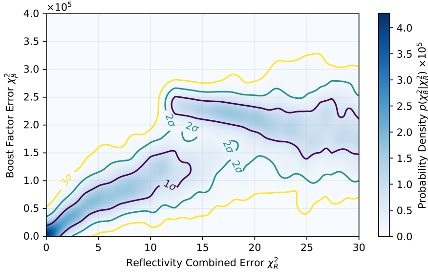
Figure 8.51: Correlation between error on the reflectivity measurement \chi_R^2 and boost factor \chi_\beta^2 . The colors denote the probability density in \chi_\beta^2 (vertical axes) for a given \chi_R^2 (horizontal axes). Assuming the distribution is approximately Gaussian, the contours show where the probability density drops to the values corresponding to 1, 2 and 3 standard deviations.
