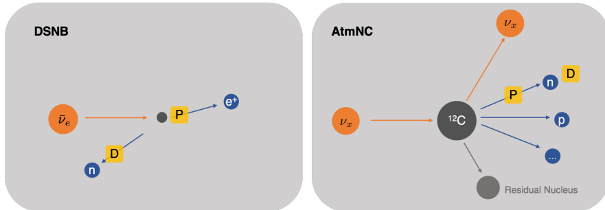
Figure 9.7: Sketch of an exemplary DSNB and atmospheric NC event. The prompt ( P ) and delayed ( D ) vertex position are closer to the reaction vertex for DSNB events than for atmospheric NC events. Since the prompt and delayed events of atmospheric NC events are caused by mainly the same neutron particle, the distance between prompt and delayed signal vertices is reduced. As the neutron and positron from the DSNB event, are in first-order emitted in opposite directions, the prompt-delayed distance is enhanced.
