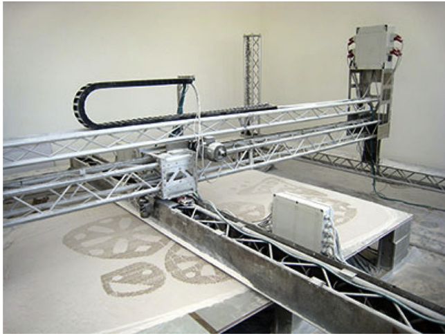
Fig. 3. Cross section produced with a D-Shape printer [55].
