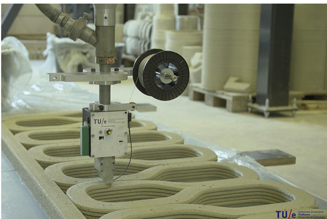
Fig. 2. 3D Concrete Printing at Eindhoven University of Technology [25].
