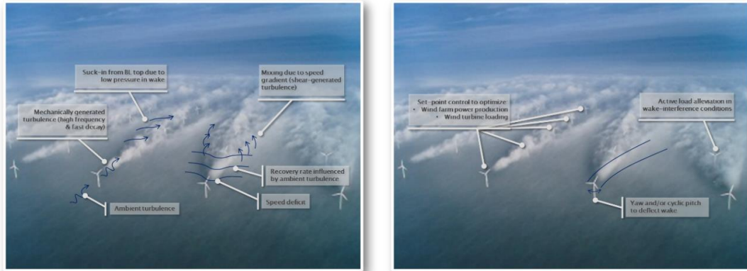
Figure 1. At left, wake and turbulence effects in a wind farm; at right: power curtailment and wake deflection strategies for wind farm cooperative control.
