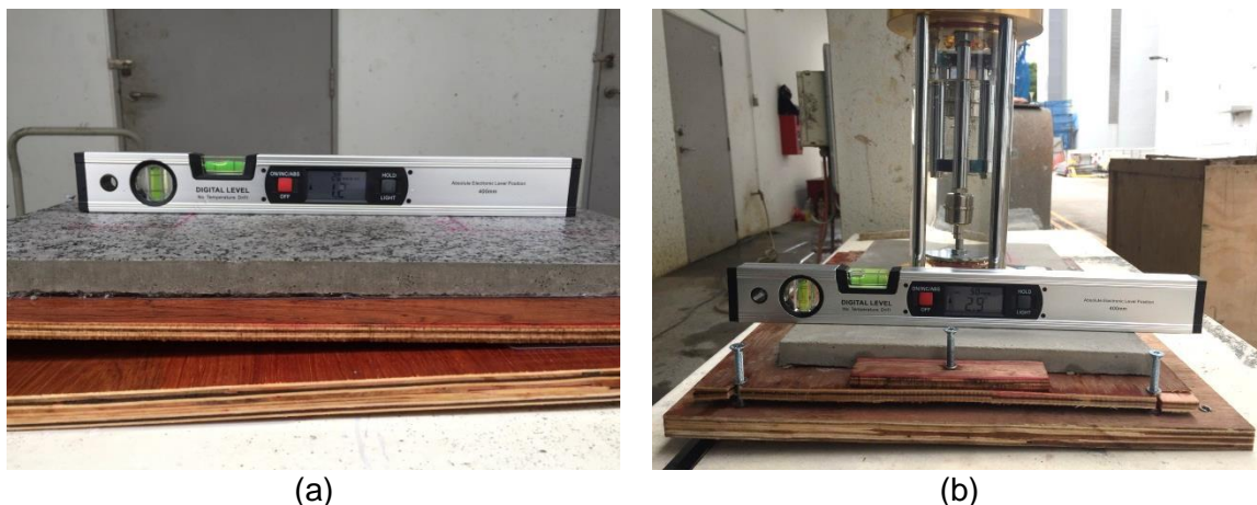
Figure 13.2 Adjustment mechanism for (a) grade and (b) cross slope of the specimen
