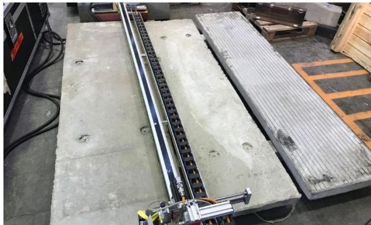
Figure 14.1 Surface profilometer measuring the texture of ECC slabs
