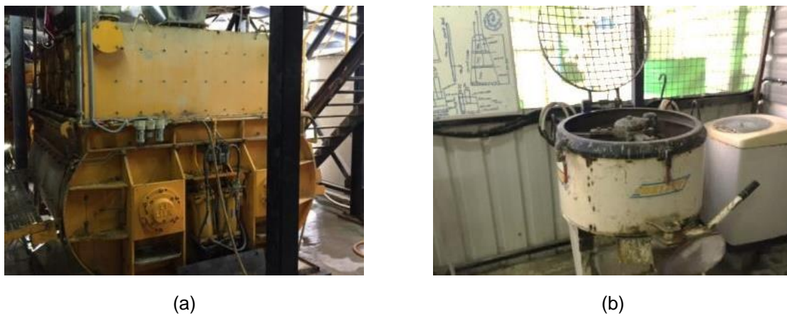
Figure 8.1 Concrete mixer (a) plant drum with 3000 L capacity, (b) with 100 L capacity
