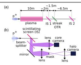
FIG. 1. (a) Schematic location of the imaging stations (IS1 and IS2) and of the OTR streak camera screen with respect to the plasma. The proton bunch moves from left to right. (b) Schematic drawing of the optical setup of the imaging stations.
