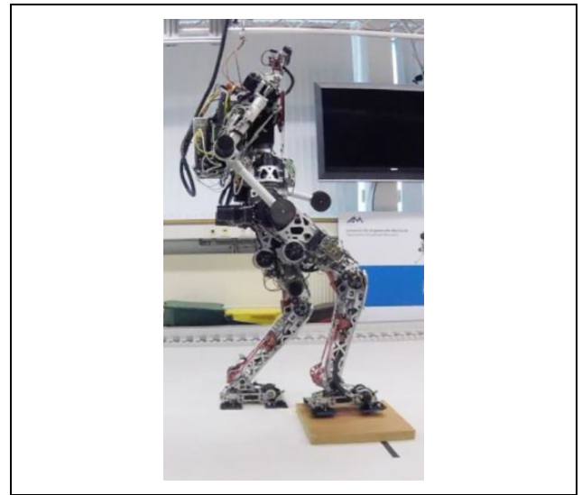
Figure 6. Experimental early-contact scenario with an undetected, 4-cm-high wooden board.
