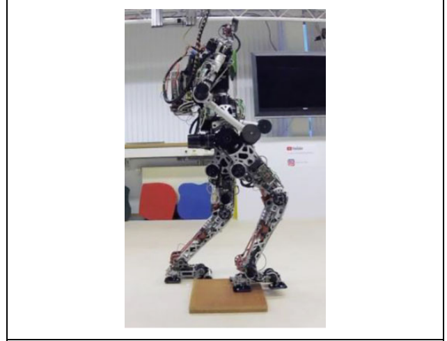
Figure 11. Experimental partial contact scenario with an undetected, 4-cm-high wooden board. The board is positioned to induce a heel-only contact of the right foot.
