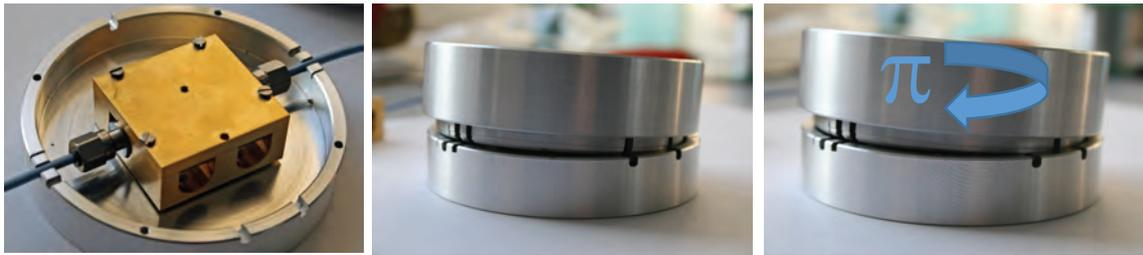
**Figure C.1:** *Magnetic screening boxes.* Panel a) mounted sample in the constructed aluminum box. Panel b) and c) show the flexibility to use the boxes either for JPA microchips (two MW input lines) or for multiplex sample geometries (up to five MW lines).
