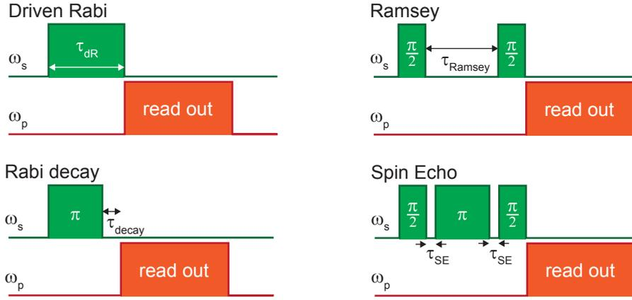
**Figure 5.8:** Applied qubit pulse schemes. Within this thesis four different pulse schemes were applied to a transmon qubit to investigate its decoherence.
