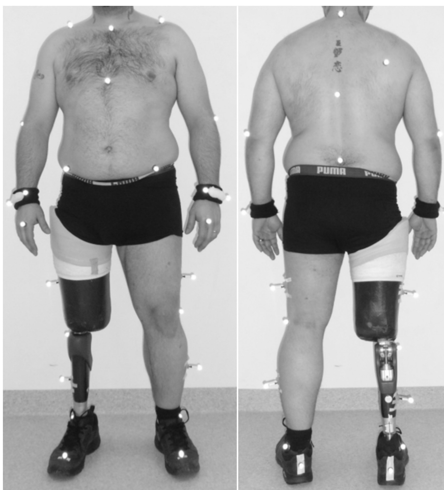
Fig. 1. Marker placement (Plug-in Gait Fullbody model). Markers on the prosthetic system were placed at the same positions as on the intact limb. Upper body: C7 (Spinous process of C7); TH 10 (Spinous process of TH 10); RBAK (Central on the right scapula); CLAV (Jugular Notch); STRN (Xiphoid process of the sternum); LSHO and RSHO (Acromio-clavicular joint left/right); LELB and RELB (Lateral epicondyle left/right); LWRA and RWRA (Process styloideus radii left/right); LASI and RASI (Anterior superior iliac spine left/right); SACR (Sacrum). Lower limbs: LTHI and RTHI (surface of the left/right thigh); LKNE and RKNE (flexion-extension axis left/right knee); LTIB and RTIB (surface of the left/right shank); LANK and RANK (lateral malleolus left/right); LHEE and RHEE (calcaneus left/right at the same height above the plantar surface of the foot as the toe marker); LTOE and RTOE (second metatarsal head).
