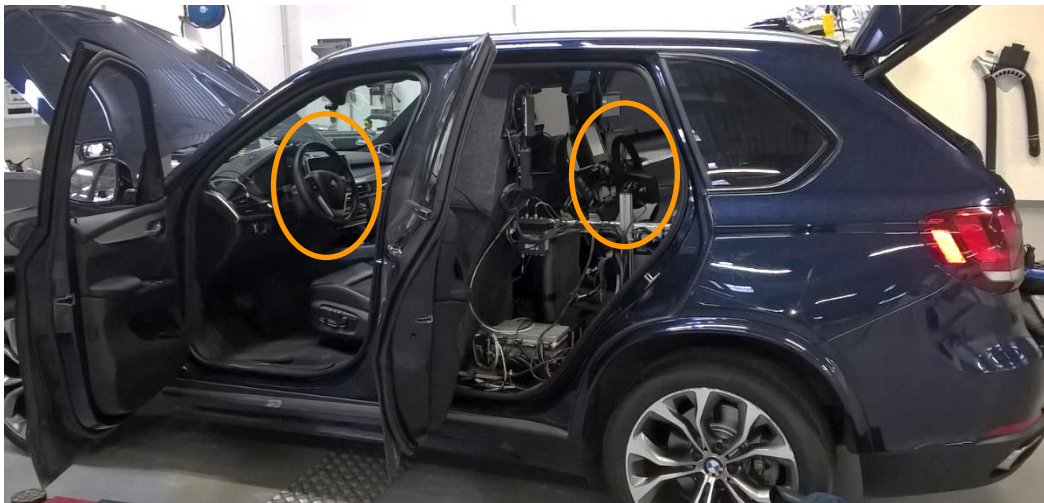
Figure 8: Wizard-of-Oz vehicle side view with the two driver workplaces.
