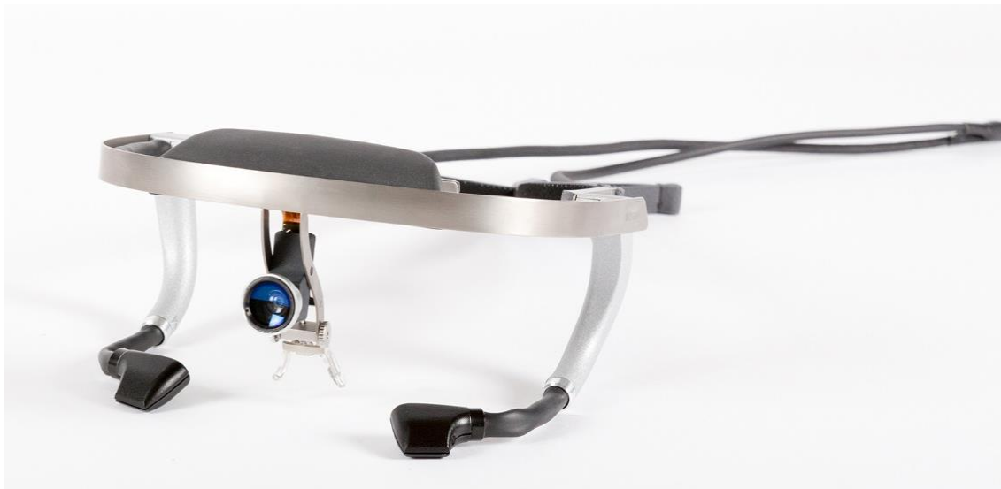
Figure 11: Dikablis Professional head-mounted eye-tracker.
