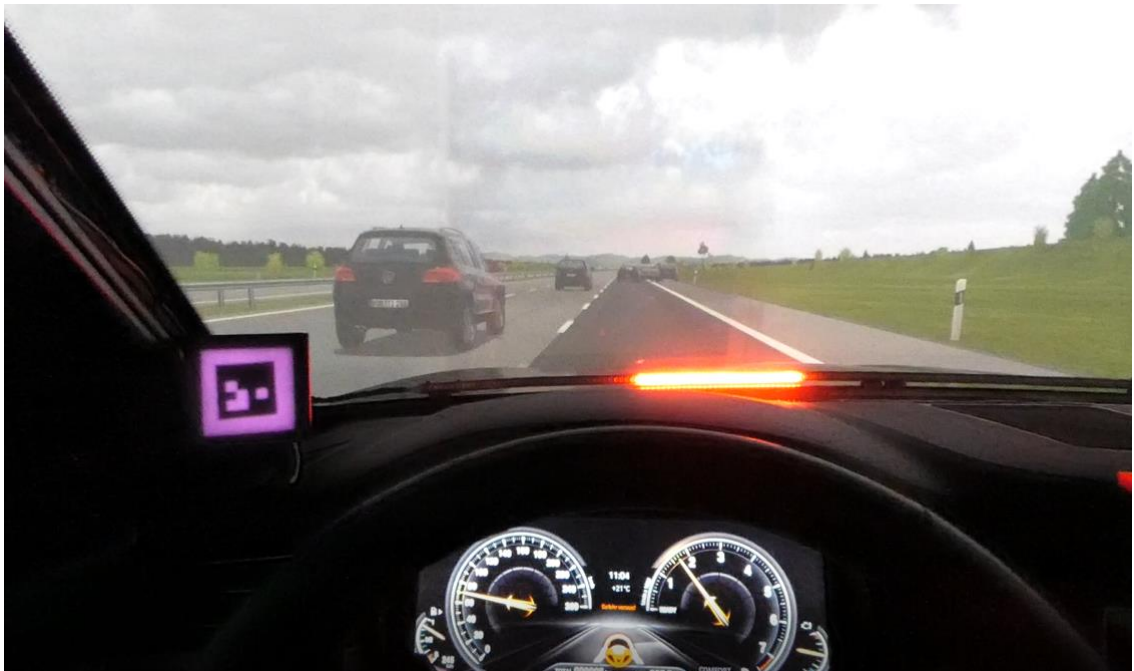
Figure 32: Experiment 4: LED light signal in the LED-concept .
