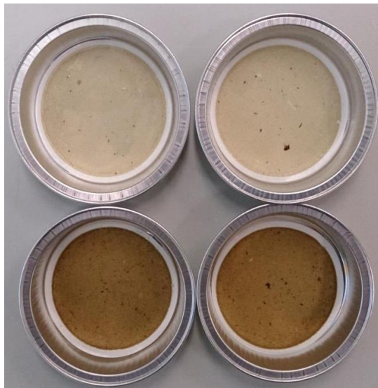
Figure 2.4: Loaded cellulose-acetate filters of the control (top) and treatment RAS (down) during the short-term exposure study (chapter 4).
