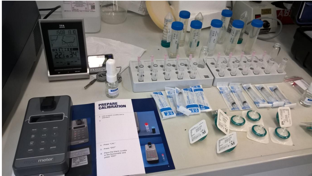
Figure 2.9: Measurement of bacterial activity using the Bactiquant® method.
