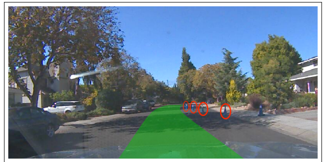
Fig. 7: Planned trajectory based on the output of the FCN path model. Part of the road is blocked by traffic cones (red circles). The trajectory is planned around them.
