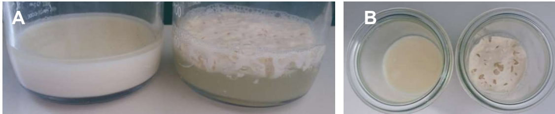
Figure 8: Influence of carbon source on the formation of LPI gels. LPI suspensions were fermented with L. curvatus TMW 1.624 and glucose (A and B, left) and sucrose (A and B, right).
