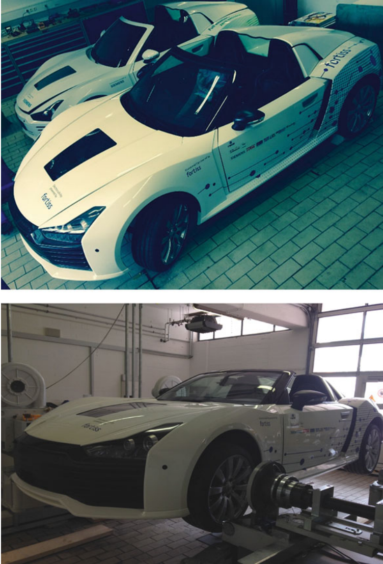
Fig. 10 The cars equipped with the RACE architecture. Top: physical appearance, bottom: car on test rig with direct coupling (all four wheels) to external electric motors that can induce very realistic driving dynamics scenarios
