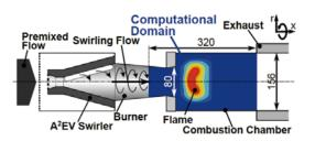
1 | Schematic of experimental combustor
