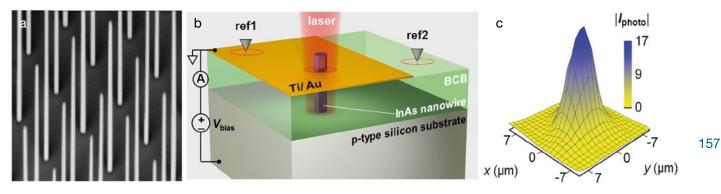
1 | (a) Site-selective In(Ga)As nanowires on Si; the optoelectronic properties of the n-InAs/p-Si heterojunction diode are probed by scanning photocurrent microscopy (b) with a typical result in (c) [1].
