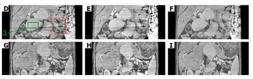
1 | Results of reconstructions from *ex vivo* mouse X-ray phase contrast CT measurements using a state-of-the-art analytical method (left), a state-of-the-art iterative method (middle), and a newly developed iterative method [3].
