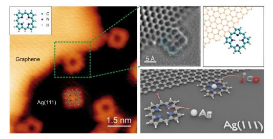
1 | Left: STM image showing porphine molecule coupled to the graphene edges (marked with green square). Right top: Laplace-filtered nc-AFM image of a porphine forming three C-C bonds with a graphene zigzag edge (left) and the corresponding structural model (right). Right bottom: Schematic model illustrating the main processes on the Ag(111) surface.
