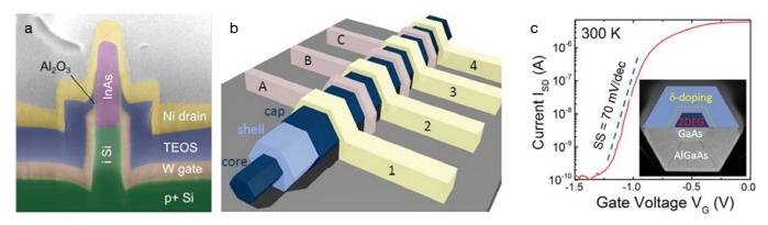
2 | (a) Vertical gate-all-around InAs-on-Si NW-TFET device [2]; (b) Multi-gated modulation-doped GaAs-AlGaAs core-shell NW-FET (b) with excellent transfer characteristics shown in (c) [4].
