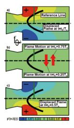
2 | Illustration of periodically displacing flame
