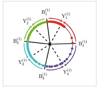
2 | Schematic representation of one step of Lloyd's algorithm in the case of 4 discrete values of the field.
