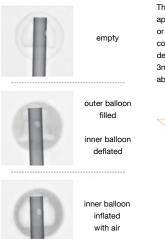
This first prototype and setup shows that an approach using Rhenium-188 for intracavitary or interstitial radiation therapy delivery that could be feasible (mainly for small tumors) for delivering a radiation boost of around 20 Gy in 3mm from the balloon surface in an acceptable time (around 30 minutes).
