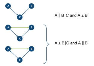
2 | Stochastic dependence (denoted by ||) and independence (denoted by ⊥) for the three fundamental connections in a Bayesian network (from top to bottom): converging connection, serial connection, and diverging connection. Single-pointed blue arrows denote stochastic dependence and green double-pointed arrows denote the associations induced by them.
