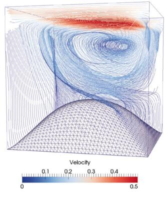
2 | Driven cavity with flexible bottom, simulated by the incompressible Navier-Stokes solver Alya (Barcelona Supercomputing Center) and the membrane solver Carat (STATIK, Technical University of Munich), coupled at runtime via preCICE.
