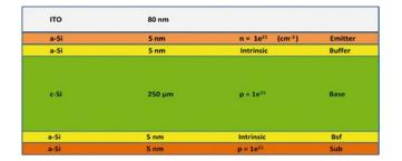
1 | Layers stack of the HIT solar cell; the light is incident from the top.
