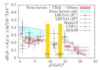
2 | Branching fraction for the rare decay  $B \rightarrow K l^+ l^-$  [3] as a function of the invariant mass of the  $l^+l^-$  system,  $q^2$ . The theoretical predictions (cyan and pink bands) lie higher than the most precise measurements from the LHCb experiment (red data points). If this "tension" is confirmed by new data and better calculations, the discrepancy would be evidence for new physical phenomena at the smallest distance scales ever probed by humankind.
