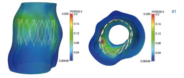
1 | Isogeometric simulation of stent implantation
