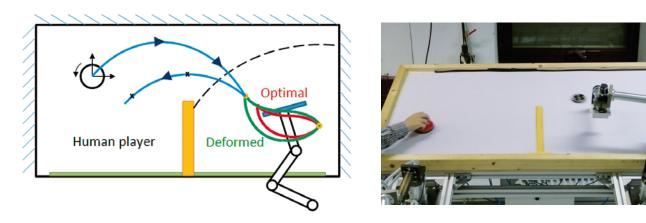
2 | Several experiments are implemented to investigate optimality and robustness of dynamic manipulation on an inclined air-table, which provides decreased gravity. The findings on trajectory deformation are tested in a planar volleyball scenario [2].
