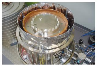
2 | TUM-Genova thermal calorimeter to measure the heat generated by the <sup>144</sup>Ce source.
