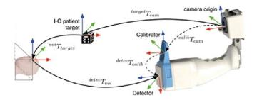
1 | Visualization of freehand SPECT reconstruction in augmented reality view. The patient target (1) is tracked and the volume of interest is rendered (2) in front of the gamma camera (3).
