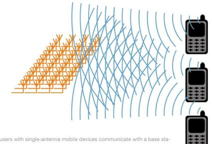
1 | Typical massive MIMO scenario: A number of K users with single-antenna mobile devices communicate with a base station that possesses a large antenna array of M antennas. M is usually an order of magnitude larger than K.
