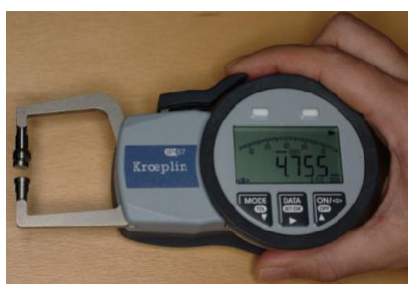
Figure 4: Measuring gauge used for measurements of ear thickness.
