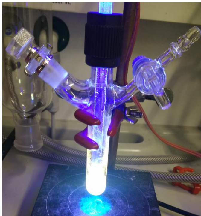
Figure 4.2. Custom-made apparatus and reaction setup for small molecule photochemistry experiments with 5 W high power LED (Avonec). The irradiation system was developed by the group of Prof. Thorsten Bach.
