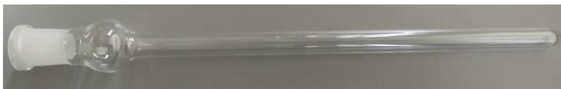
Figure 4.1. Custom-made phototubes used for photolysis reactions performed in Rayonet photoreactors.
