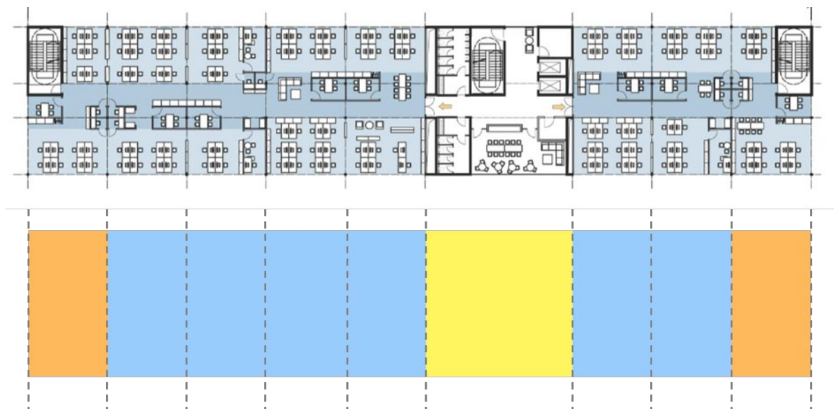
Figure 27 Core unit (yellow), office units (blue) and seam units (orange) in a standard ConEx layout
