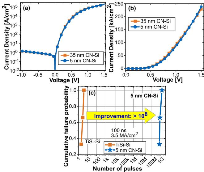
**FIGURE 12.** Comparison of the dc characteristics of CN-Si diodes with 5 nm and 35 nm thick CN in a semi-log (a) and linear (b) scale. Both curves almost match each other. (c) compares the failure probability of the 5 nm CN-Si to the TiSi-Si diodes under the same test conditions (100 ns, 3.5 MA/cm<sup>2</sup>). The devices failed the reliability test within a window of 660 million to 1.28 billion pulses.
