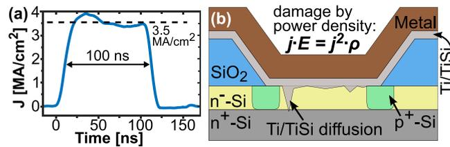
**FIGURE 2.** (a) A measured waveform of a 100 ns current pulse with a rise/fall time of < 15 ns and an average current density  $j = 3.5 \text{ MA/cm}^2$ , which was measured with a Tektronix CT-1 current sensor. (b) Schematic cross-section of a TiSi-Si Schottky diode where Ti or TiSi diffuses into the n<sup>-</sup>-Si epitaxial layer and could even reach the highly doped substrate by the application of high current pulses. Adapted from [11].
