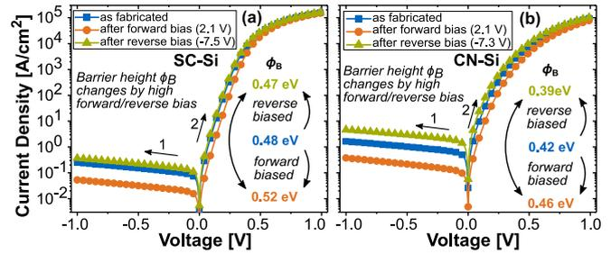
**FIGURE 6.** Comparison of the dc-characteristics of a SC-diode (a) and a CN-diode (b) as fabricated, after being forward biased with 2.1 V and after being reverse biased with 7.5 V or 7.3 V, respectively. The reverse characteristics were measured before the forward direction at the illustrated curves. The SBH  $\phi_B$  changes according to the applied polarity and is reversible by applying the opposite polarity.
