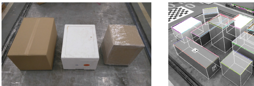
Fig. 9. Test boxes used and tracking of multiple boxes in a pallet
