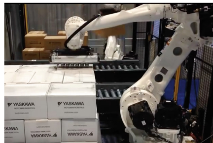
Fig. 2. SICK LMS Line Scanning and Universal Robotic's Depalletization
