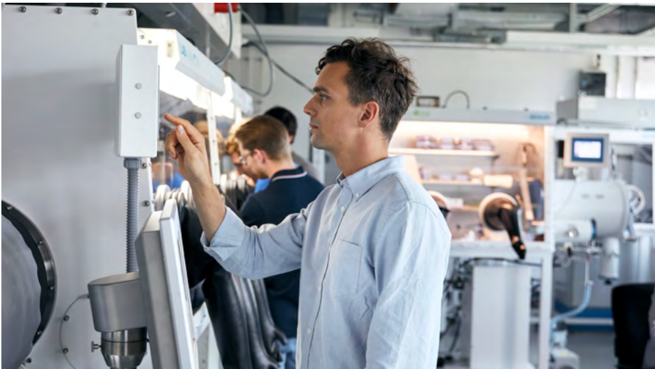
■ View into the ZEI battery lab with glove boxes for pouch cell manufacturing in the background
