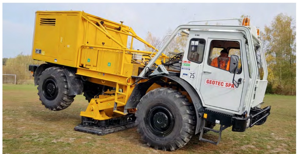
■ Vibro-truck during 2D-seismic campaign. The reflected signals are collected by geophones and reprocessed later. Source: Geothermal Alliance Bavaria, FAU.
