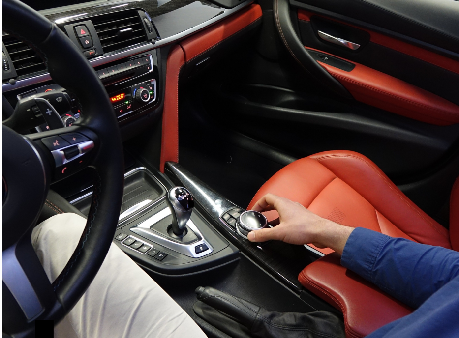
Figure 6.2: Rating knob for the CR located on the central console of the mockup.
