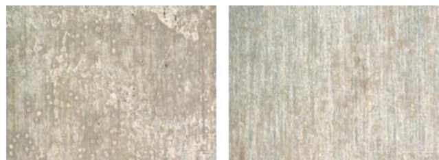
Figure 6: Aluminium samples without (left) and with 2 plasma coating passes (right) after 48 h immersion in 5% NaCl solution.
