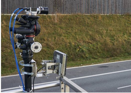
Fig. 3: Our sensor setup with a radar and camera above the highway.
