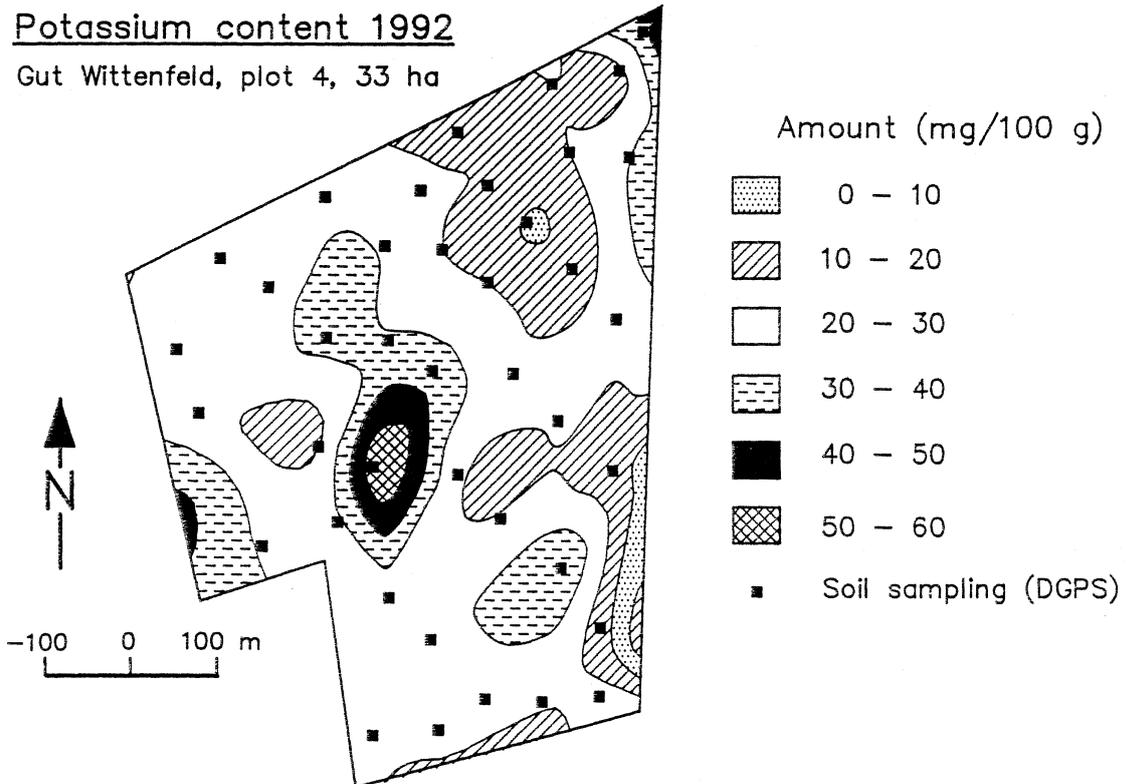
Fig. 5: Graduated potassium supply with respect to geo-referenced soil sampling.
