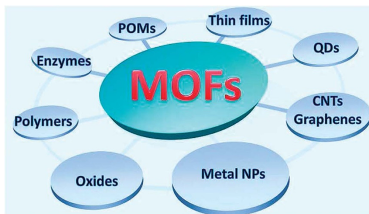
Figure 1.5. The composites of MOFs and functional materials. [Reprinted with permission from ref. 49. Copyright 2014 The Royal Society of Chemistry]
