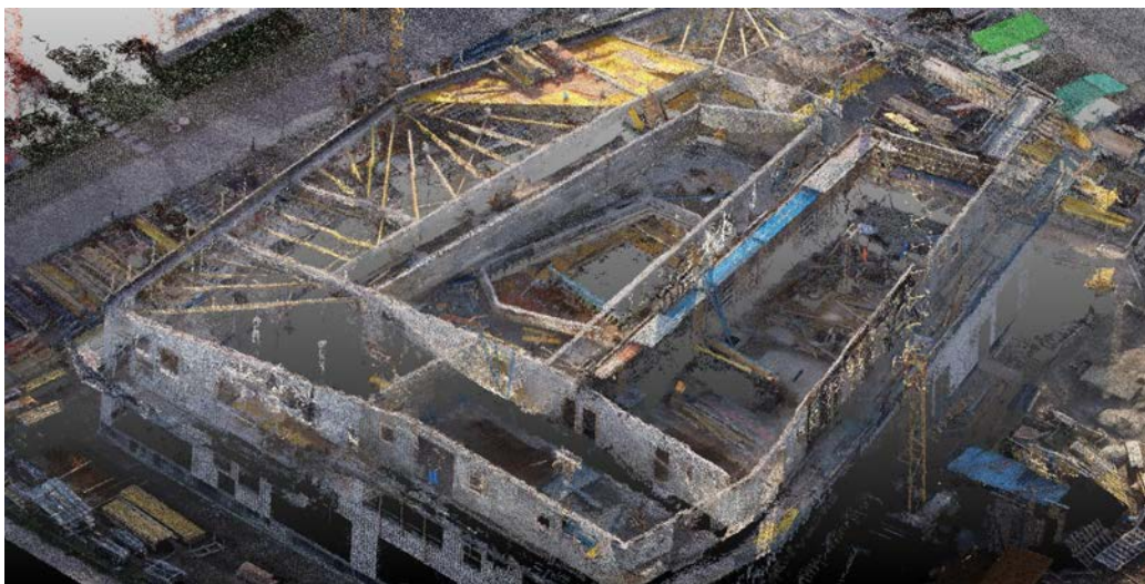
Figure 2: Occluded construction elements in generated point cloud caused by scaffolding, formworks, existing elements and missing information during the reconstruction process
