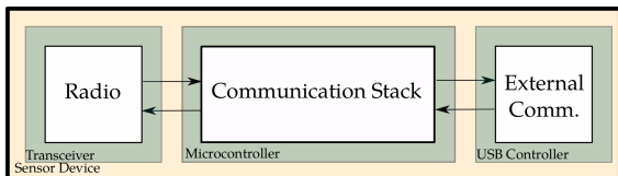
Fig. 1: Different computation units on a typical sensor device. Transceiver does wireless reception while the USB controller handle forwarding of the packet where both have to share the microcontroller resources.
