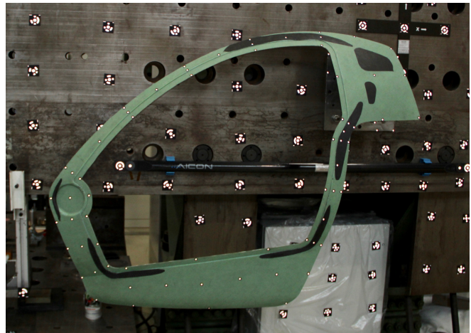
Fig. 9. Experimental Setup for Static Load Tests on Built Hybrid Cabin Door
