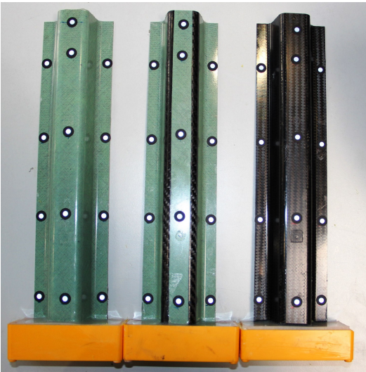
Fig. 6. Photograph of Epoxy Embedded Beams from Left to Right: Flax, Hybrid, Carbon
