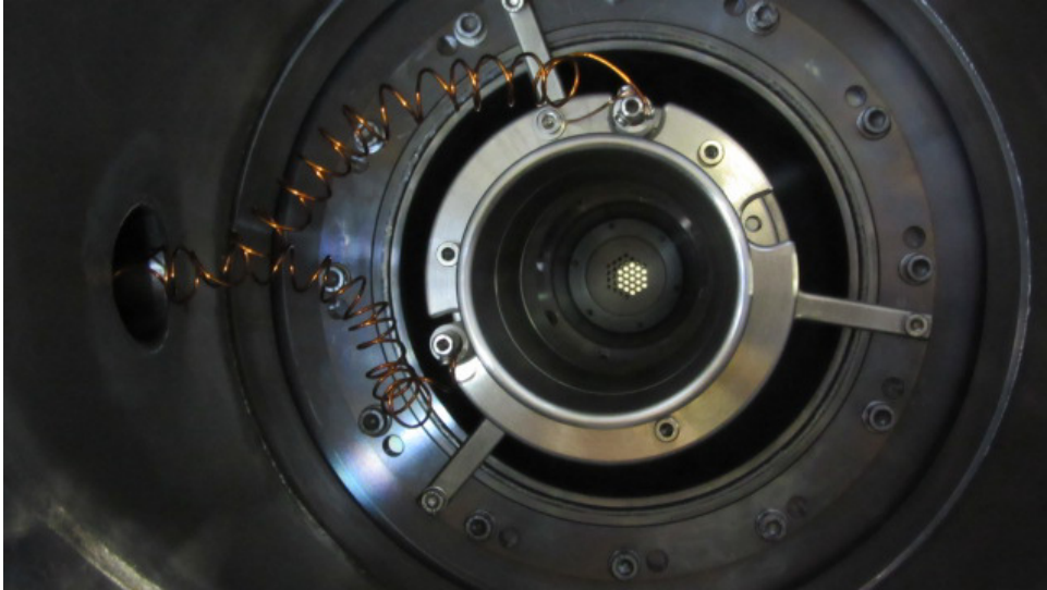
Figure 4.30: Einzel lens installed in the first differential pumping stage at the exit of the ion source, marked 1st einzel lens in the bird's-eye view of SIESTA (Fig. 4.1).
