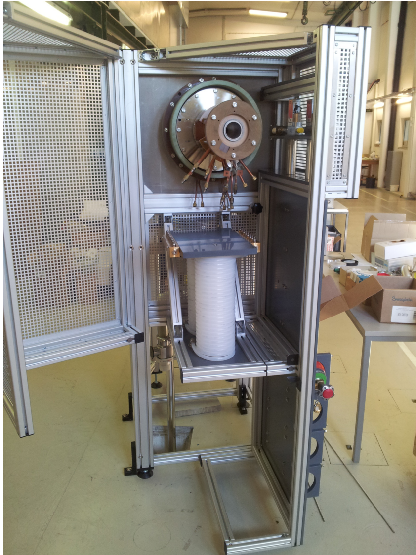
Figure 4.4: High-voltage cage of the DuopIGatron ion source. Below the source, the cooling lines coiled into double spirals can be observed.
