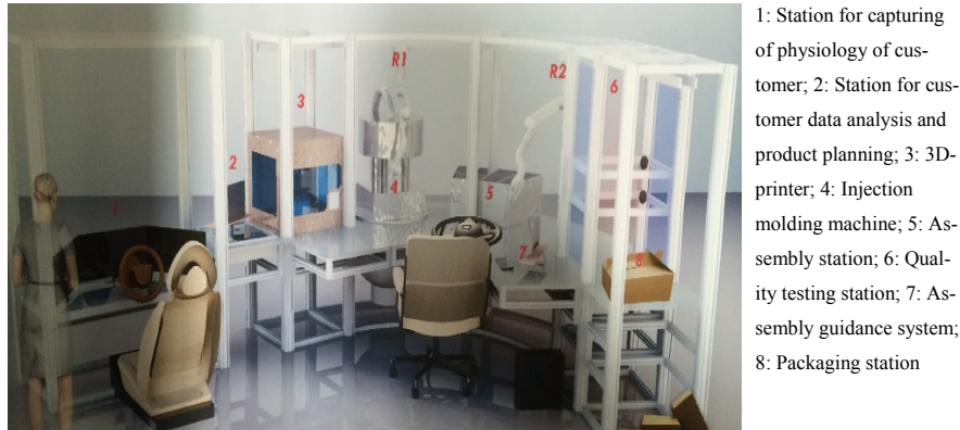
Fig. 8: Setting for the design and production of personalized automotive equipment (in this case a personalized steering wheel)
