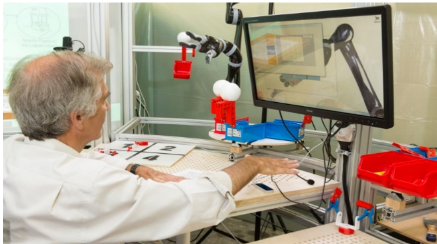
Fig. 2: Elderly person producing a personalised product by a collaborative robot system that is informatically and kinematically integrated with the workstation.
