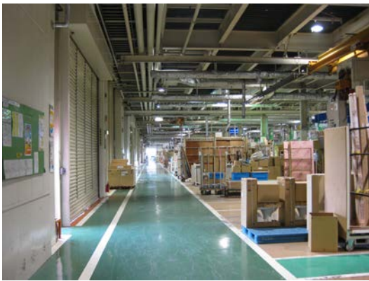
Figure 3: Interior view of one of the two supply sides which flank the production line. The components and materials are supplied from the left side just in time and just in sequence to a small “preparation” area which can be seen on the right side. The preparation area is located next to the production line. Sekisui Heim.
