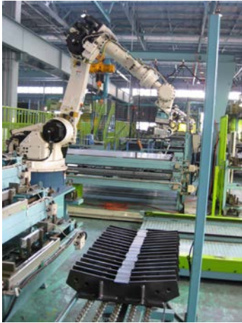
Figure 2: Robots position various steel components automatically to onto a laying table for frame elements. The laying table then carries the frame into the automatic welding station. Thus every 3-5 minutes a new basic frame element is generated.
