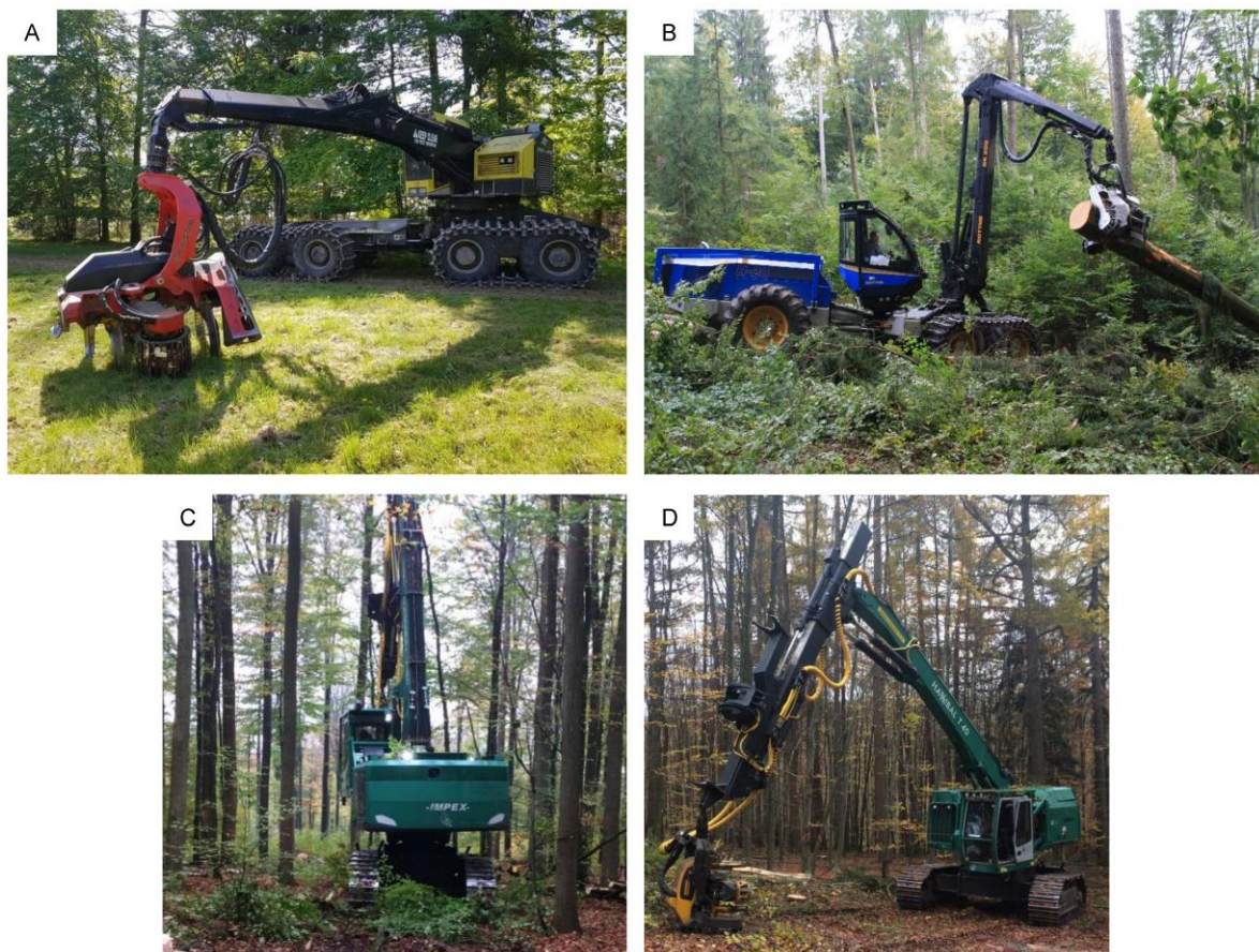
Figure 1. Harvesters used in the study: (A) TimberPro TF840-B, (B) Rottne H20, (C) Impex Hannibal T50, and (D) Impex Hannibal T40. Photo credit: (A) [16]; (B–D) [17].
