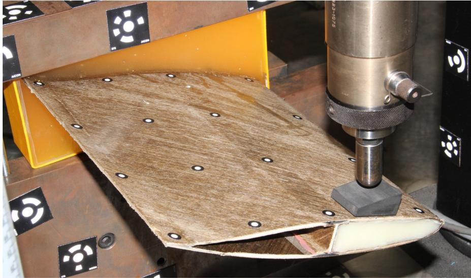
**Fig. 5** Experimental setup of cyclic loading in a cantilever beam with force application angle of  $18.7^\circ$
