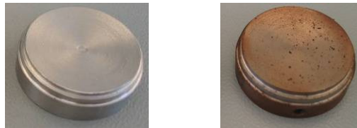
Fig. 5: Image of the diffuse reflector before (left) and after (right) deployment of the sensor in an oil furnace for one month.
