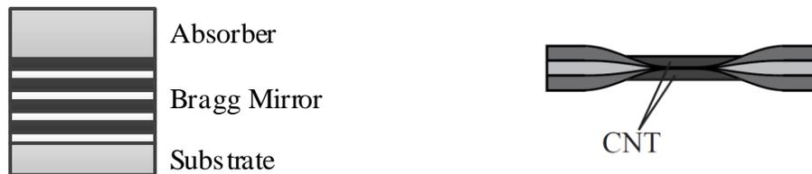
**Figure 2-13: Scheme of (a) a SESAM absorber and (b) a tapered fiber carbon nanotube absorber.**
