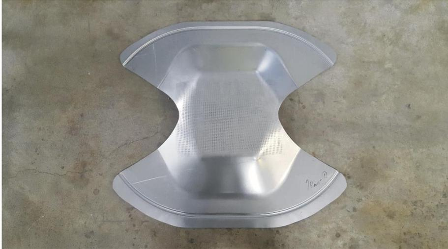
*Figure 9.2: a preformed part for HX260LAD as example*
