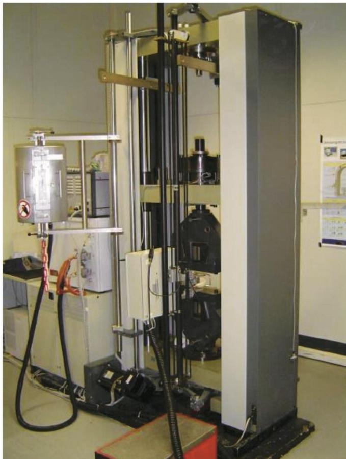
Figure 4.1: Universal test machine 200 kN
