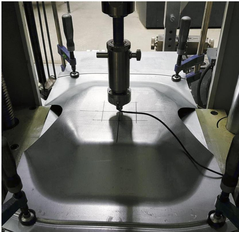
*Figure 9.9: Stiffness test for loading on the middle of the part*
