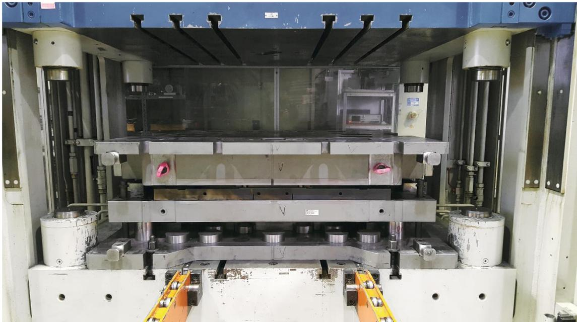
*Figure 9.1: installed entire tools for preforming and bead forming in hydraulic press*
