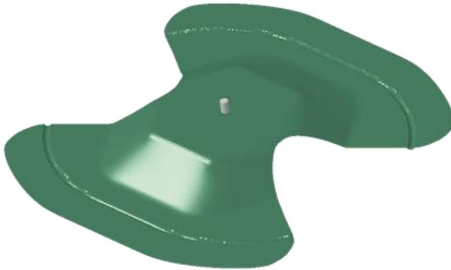
*Figure 7.10: Stiffness analysis in the forming simulation using pin loading on the middle of the part*
