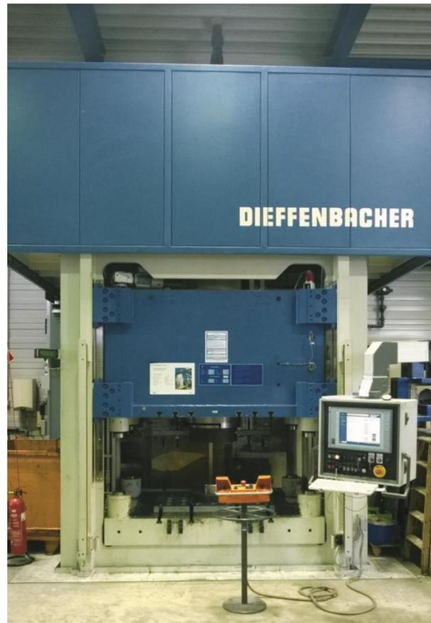
*Figure 4.5: Diffenbacher hydraulic press*
