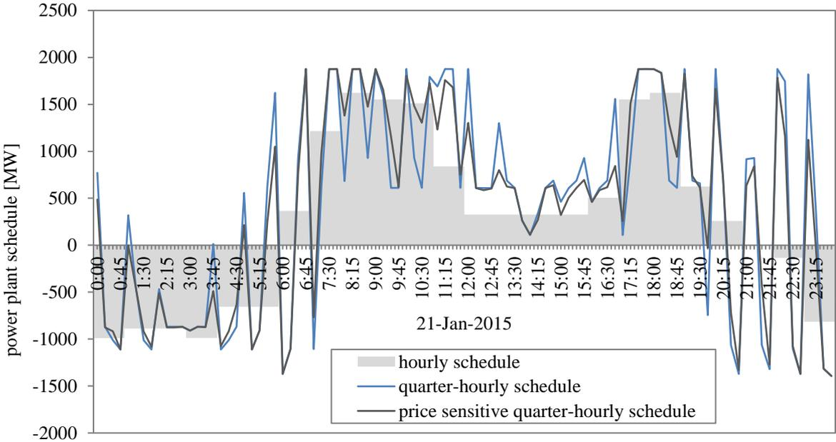
Figure 52 Comparing the production schedule of the first stage optimization for the hourly day-ahead auction (yellow bars) with the production schedule of the post-optimization for the quarter-hourly day-ahead auction (blue line) and considering price sensitive (red dotted line)
