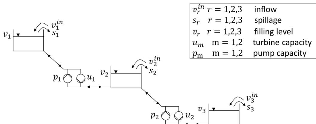
Figure 66 Reservoir cascade with three reservoirs connected with turbines and pumps
