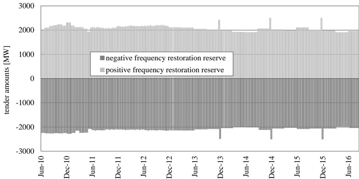
Figure 20 FRR demand of the German TSOs or the group of TSOs in which the German TSOs is organized. Data derived from (Regelleistung.net, 2017a)
