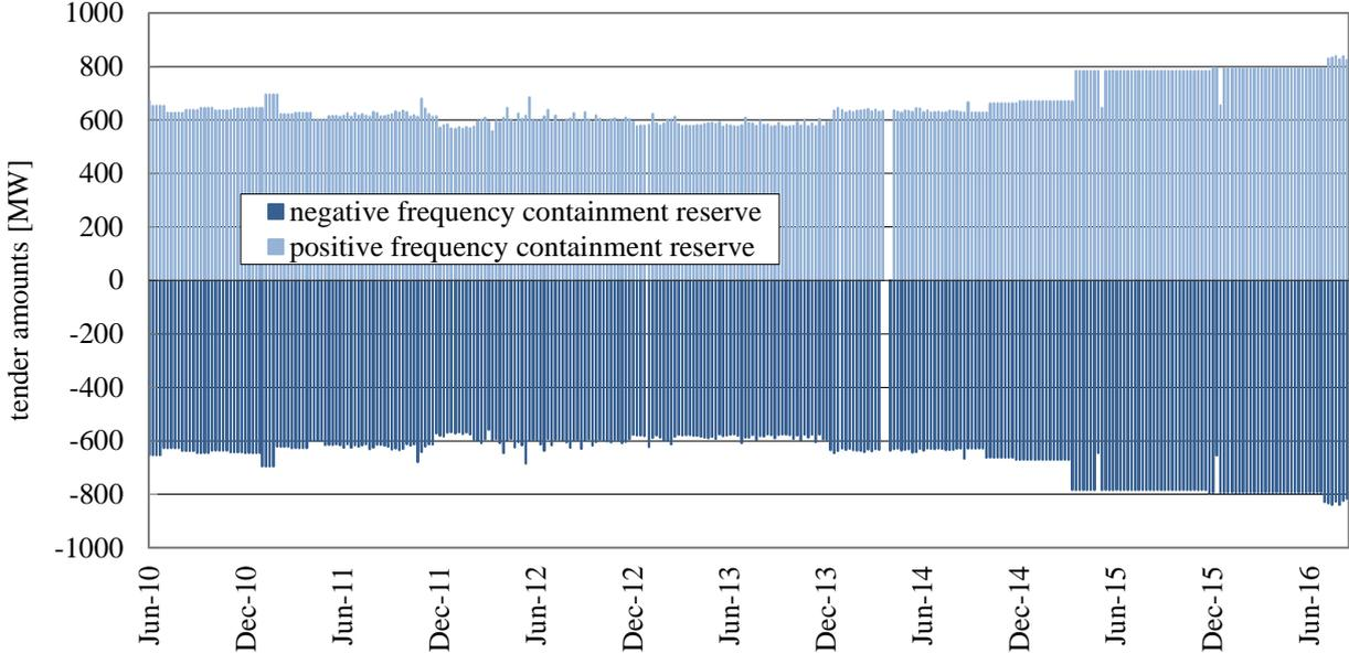
Figure 18 Positive and negative FCR demand of the German TSOs or the group of TSOs in which the German TSOs is organized. Data derived from (Regelleistung.net, 2017a)
