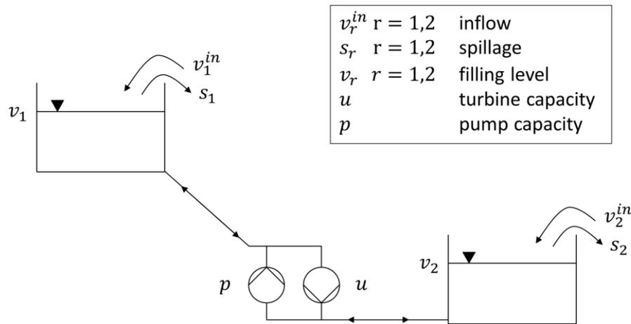
Figure 35 Diagram of a pumped hydropower storage with two reservoirs
