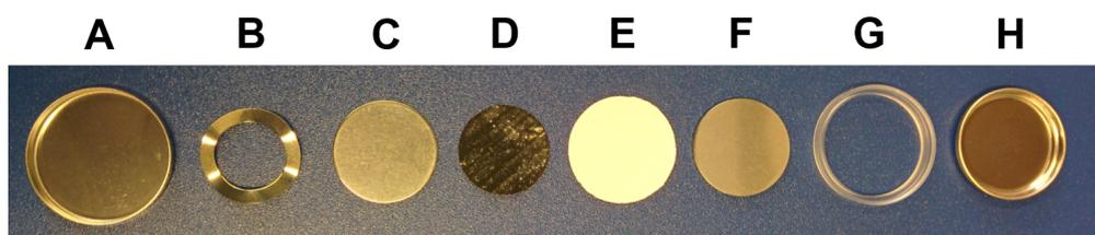
**Figure 1.2:** List of parts required to build a coin cell battery half cell. **A:** Stainless steel lid, **B:** Stainless steel spring, **C:** Stainless steel spacer, **D:** Anode prepared as described above, **E:** Glasfiber separator saturated with electrolyte, **F:** Lithium or sodium cathode, **G:** Gasket, **H:** Stainless steel bottom.
