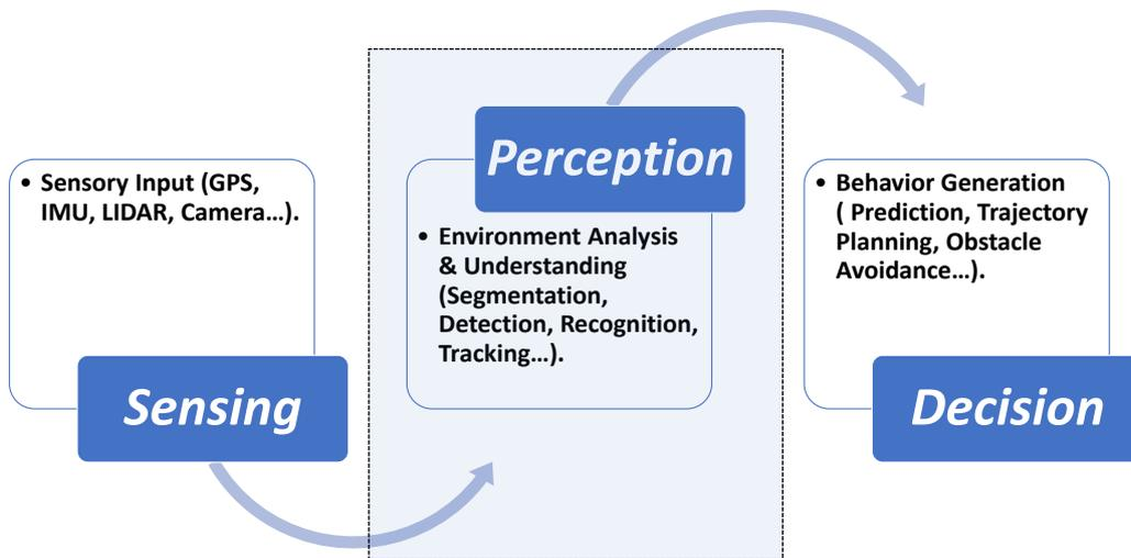
**Figure 1.2:** The flowchart of the full autonomous driving process (Level 5).
