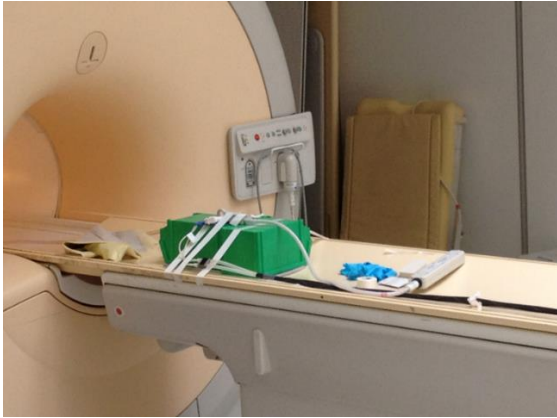
Figure 8: MR imaging setup using a human MRI system: The mouse was anesthetized with isoflurane and taped to boxes to avoid motion artifacts. A tail vein catheter allowed for contrast agent injection between the MR sequences. A surface coil was placed above the hind legs to improve MR image quality.
